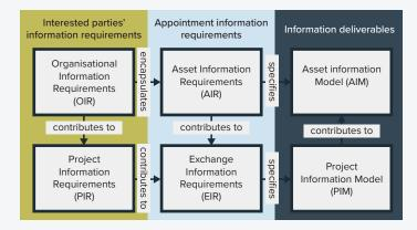
NOTE: In this figure, 'encapsulates' means 'provides the input to', 'contributes to' means 'provides an input to', 'specifies' means 'determines the content, structure and methodology'. BUILT ASSET INFORMATION MANAGEMENT
